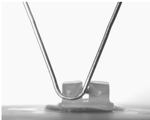
FIGURE 3. A 0.014-inch steel ligature wire looped under the distoincisoral tie wing for tensile testing.
