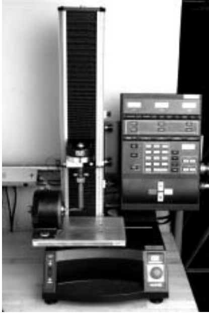
Figure 8. The Instron test machine measures torque strength of an Inspire bracket by placing a load to the end of a key that torques the wire ligated in a bracket.
